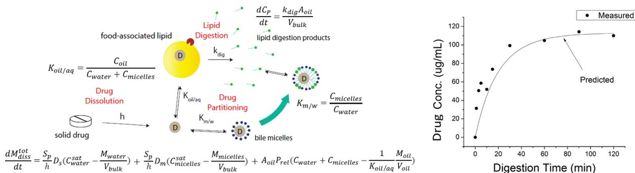
Figure 1: Left - Schematic of proposed mechanism of ingested lipid impact on drug behavior in the GI tract and respective equations. Right - Measured vs. predicted carbamazepine dissolution profile during a multi-process experiment including lipid digestion and drug partitioning.
