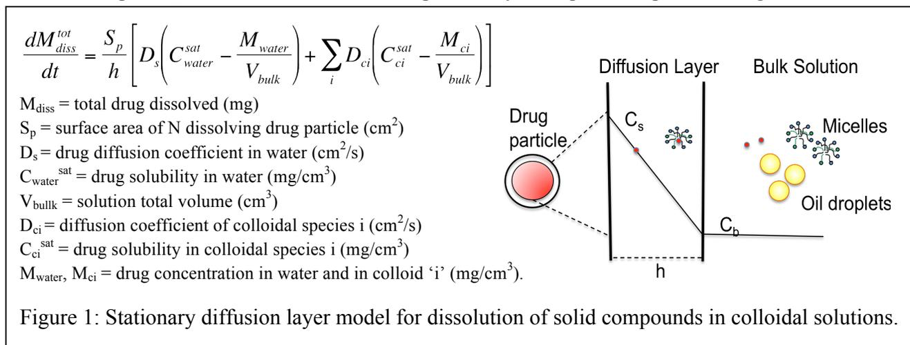
Figure 1: Stationary diffusion layer model for dissolution of solid compounds in colloidal solutions.
